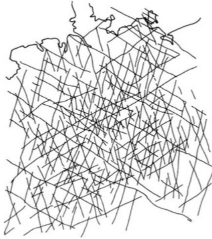
Figure 8.1 Distribution of linear fault zones in Central Europe (from Weber, 1977). The system of lines can be interpreted as a sample of a planar fibre process. A line process could also serve at least as a rough approximation; the pattern can be also interpreted as a sample of a geometrical network. Note that some of the fault zones end at other fault zones – so clearly there is interaction between them. The structure is clearly not isotropic. There are four dominating directions, ENE–WSW, NNE–SSW, NW–SE, ESE–WNW. The apparent lower intensity of fault zones in the northern region of the figure is due to incomplete information about that region. See the statistical analysis of fault lengths in Section 6.6.4, Figure 6.16.
