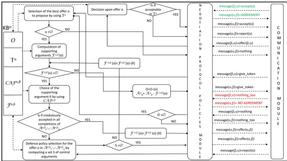
Fig. 6 Architecture of a negotiating agent  $\alpha$
