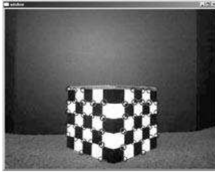
Figure 3: Automatic edge detection selects the corners of the calibration cube. Any circled edge can be selected as a calibration point.
