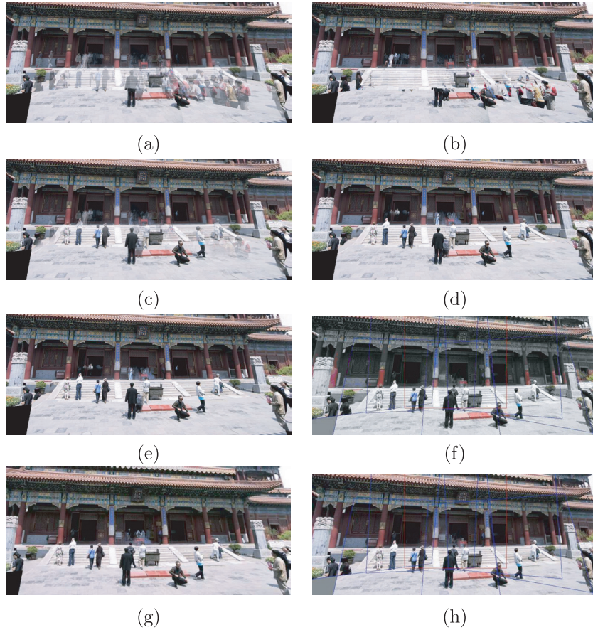
Fig. 6.1 Final composites computed by a variety of algorithms: (a) average, (b) median, (c) feathered average, (d) p -norm p = 10 , (e) Vornoi, (f) weighted ROD vertex cover with feathering, (g) graph cut seams with Poisson blending, (h) and with pyramid blending.
