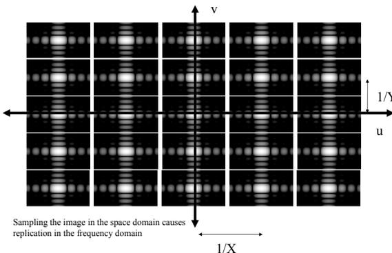
Sampling the image in the space domain causes replication in the frequency domain
