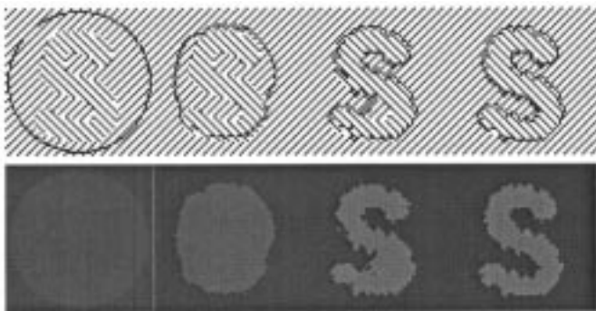
Fig. 16. Grouping based on orientation identity. In our model, we replaced u_0 from Fig. 14 bottom left, by the orientation of the normal to the level curves of u_0 (Fig. 14 bottom right). Size: 64 \times 64 , \mu = 0.025 \cdot 255^2 , \nu = 0.02 \cdot 255^2 , \phi_0(x, y) = -\sqrt{(x - 32.5)^2 + (y - 32.5)^2} + 30 , five iterations of reinitialization, \text{cpu} = 10.25 s.
