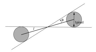
Figure 8.3: Uncertainty cone of a line segment [Shu99]. The position of the endpoints of a length l segment has a half-pixel error margin. Hence the supporting line of this segment lies within an uncertainty cone centered at the segment barycenter with angle  $d\theta = \arcsin \frac{1}{l}$ .
