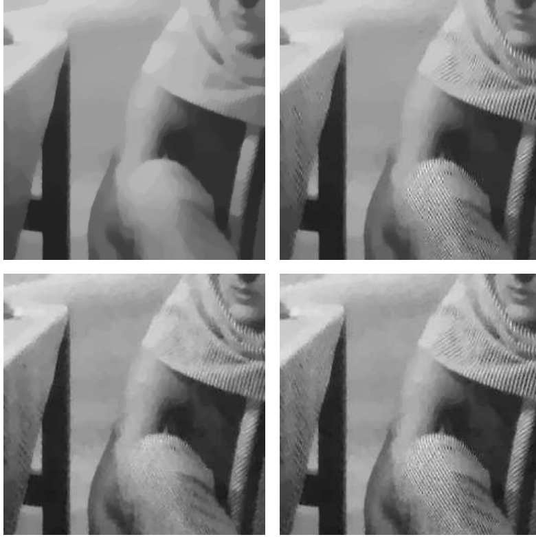
FIGURE 4. Image denoising with different values of \lambda (top line: \lambda = 0.02 , bottom line: \lambda = 0.05 ). Left column: ROF Model; Right column: our model.
