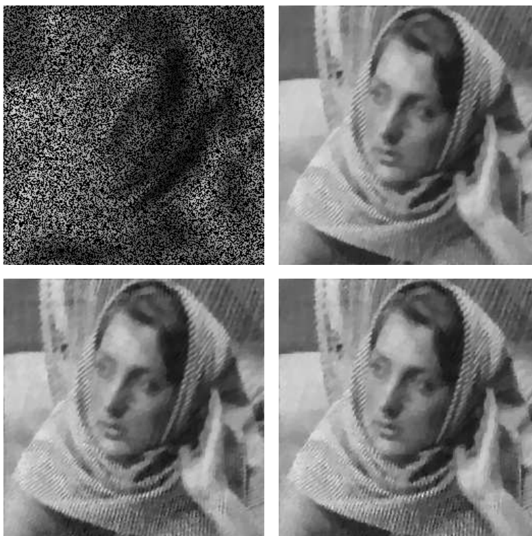
FIGURE 12. Image inpainting with randomly missing pixels. Top, left: corrupted image; Top, right: ROF model (993 iterations, CPU time=142s, PSNR=24.29dB); Bottom, left: LM model (2449 iterations, CPU time=2477s, PSNR=24.63dB); Bottom, right: Proposed model (1856 iterations, CPU time=2084s, PSNR=25.06dB).
