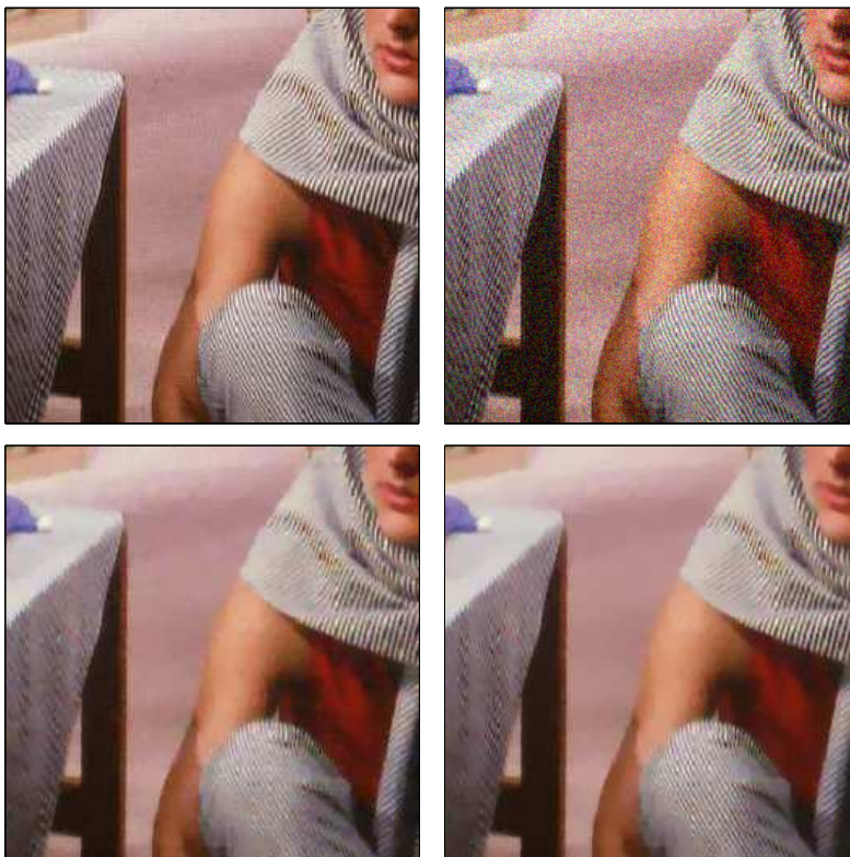
FIGURE 7. Color image denoising. Top, left: original color image; Top, right: noisy image; Bottom, left: vectorial ROF model (480 iterations, CPU time=10.7s, PSNR=26.54dB); Bottom, right: Proposed model (238 iterations, CPU time=626.2s, PSNR=26.92dB).
