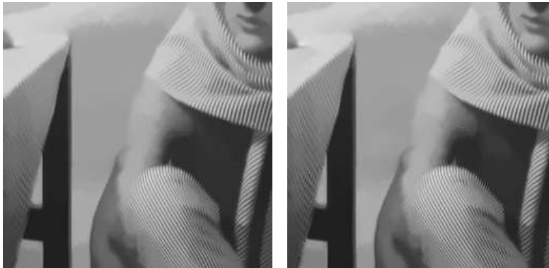
FIGURE 15. Image denoising based on NLTV regularization. Left: NLTV restoration model (PSNR=28.11dB); Right: Proposed model (PSNR=28.68dB).
