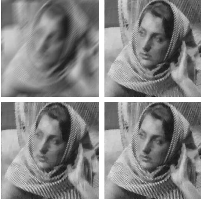
FIGURE 10. Restoration from motion blur. Top, left: blurred image; Top, right: ROF model (806 iterations, CPU time=8.1s, PSNR=25.58dB); Bottom, left: LM model (3348 iterations, CPU time=3402s, PSNR=26.21dB); Bottom, right: Proposed model (1546 iterations, CPU time=1382s, PSNR= 27.14dB).
