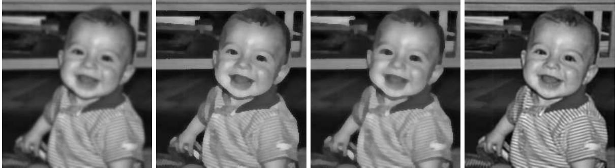
Figure 8: Image deblurring by shock filters and by a variational method. From left to right : blurred image, Rudin-Osher shock filter [30] which is a pseudoinverse of the heat equation attaining a steady state, Kramer’s [21] improved shock filter, also attaining a steady state and the Rudin, Osher, Fatemi [30] restoration method, obtained by deblurring with a controlled image total variation. This last method is very efficient when the noise and blur models are known. It is currently being used by the French Space Agency (CNES) for satellite image restoration.
