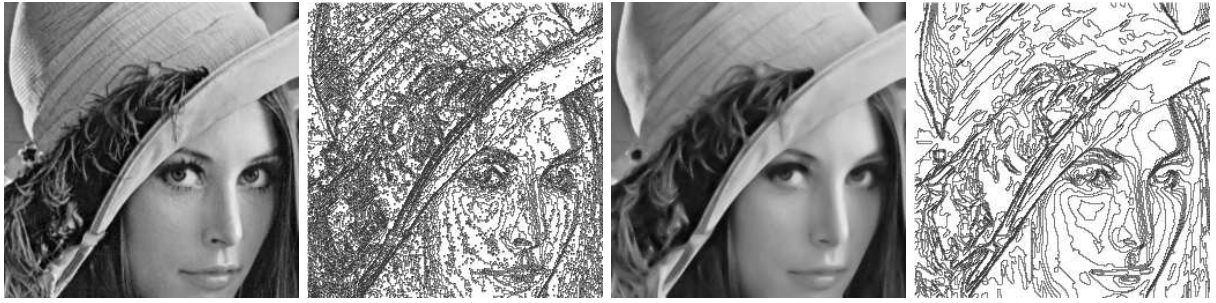
Figure 19: The Affine and Morphological Scale Space (AMSS model). From left to right : original image, level lines of the images (16 levels only), smoothed image by using the affine and morphological scale space, and its level lines.
