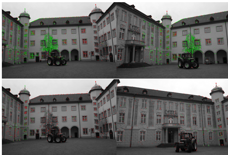
Fig. 2. Pairs (0,1) on top and (0,4) on bottom of the used Strecha’s Castle-P19 sequence. For visualization purposes, the data matches were classified as inliers (green) and outliers (red) using an arbitrary threshold of 3 pixels on groundtruth errors.
