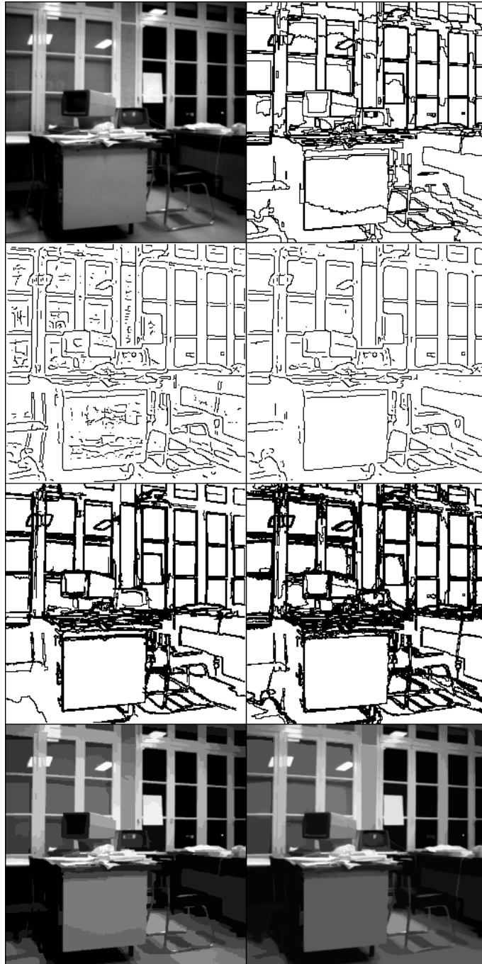
Figure 2. First row: left: original image; right: boundaries obtained with the Mumford-Shah model (1000 regions). Second row: edges obtained with Canny-Deriche edge detector, for two different threshold values (2 and 15). Third row: edges (left) and boundaries (right) obtained with our model ( \varepsilon = 1 ). Fourth row: reconstruction with the Mumford-Shah model (left) and with our model (right). This last reconstruction is easily performed by the following algorithm: attribute to each pixel x the level of the smallest (for inclusion) meaningful level line surrounding x (see (Monasse, 1999)).
