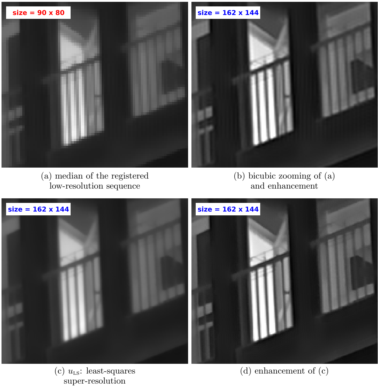
Figure 17: Effect of the enhancement filter \psi_5 on the super-resolved image. We consider again the thermal infrared sequence u_0 of L = 500 low-resolution images with size 200 \times 200 (see Section 5.5 and Figure 12). We display in (a) a 90 \times 80 close-up of the shift-and-median reconstruction (that is, the pointwise median of the registered sequence of low-resolution images). By magnifying this reconstruction with a factor 1.8 in both directions (bicubic zooming) we get an image with size 360 \times 360 on which we apply the enhancement filter defined by \psi_5 , leading to the close-up image (b). We can see that the enhancement yields an image with better contrast and a better level of details, but at the same time, amplified artifacts. We display in (c) and (d) equivalent close-ups for the least-squares super-resolution image u_{LS} obtained from u_0 (zoom factors: z_x = z_y = 1.8 ). It is interesting to see that the enhancement of u_{LS} , in addition to its ability to better reveal super-resolution details, does not produce any noticeable artifact.
