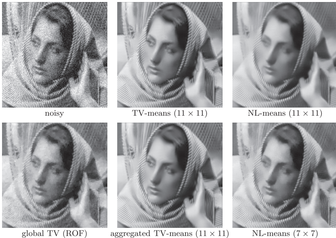
Figure 8. Denoising of Barbara image (detail). The classic Barbara image, corrupted with a Gaussian white noise with standard deviation \sigma = 20 (top left), is denoised using several methods compared in this paper. The ROF method (bottom left) does not manage to handle well the smooth and textured parts: most textured parts (scarf, basket chair) are poorly reconstructed, while a nonnegligible amount of noise remains in the originally smooth regions (cheek, hand). The NL-means method (right column, top and bottom rows) performs better, but some regions are oversmoothed (eye, basket chair) due to the patch-jittering effect mentioned at the end of section 7.1. This effect is particularly strong for 11 \times 11 patches (top row); it can be reduced by using smaller patches ( 7 \times 7 in bottom row), which leads to a better image but with a noticeable loss of denoising in some parts (hand, cheek). The TV-means algorithm we propose (middle column) manages to find an interesting compromise: it avoids the patch-jittering effect without reducing too much the amount of denoising in other regions, thanks to the use of local TV-denoising. The aggregated version (middle column, bottom row) yields a balanced restoration, visually nicer and significantly better than other methods in terms of the peak signal-to-noise ratio (PSNR) (see Table 1). Note that all images above were enhanced by a same affine contrast change for an easier visualization.
