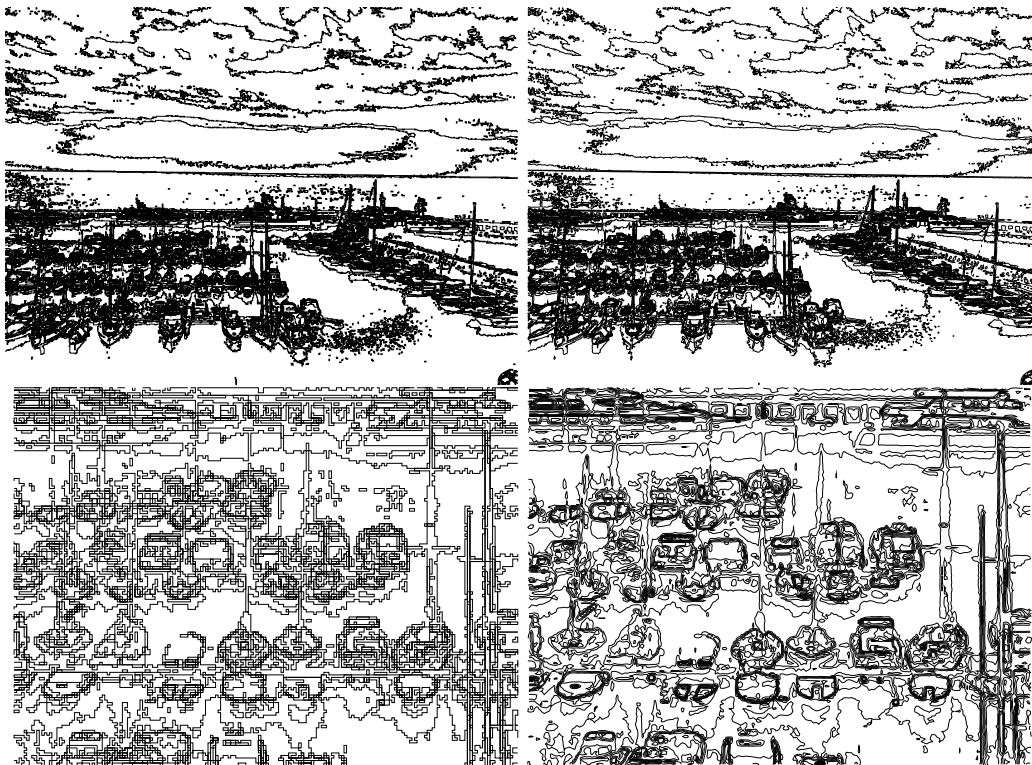
Figure 3.8: Some level lines of the left image of Figure 3.1. Left column : nearest neighbor interpolation. Right column : bilinear interpolation. The finest scales (down) reveal the superiority of the bilinear interpolation over the zero order model. Another important improvement would probably be realized with higher order splines.
