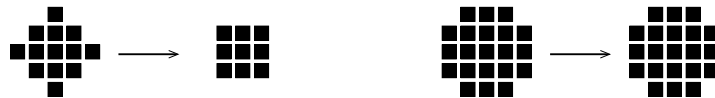
Figure 5.2: The 3 \times 3 median shrinks a discrete disc with radius 2, but has no effect on a disc with radius \sqrt{5} .
