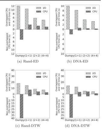
**Fig. 20** Parallel exact search time with DumpyOS. The first column is for single-thread Dumpy and the rest three columns are for DumpyOS. On x-axis, A + B indicates A threads for reading, and B threads for computing
